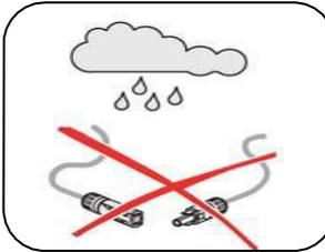
Do not fit solar modules and wiring with wet plugs and sockets!
