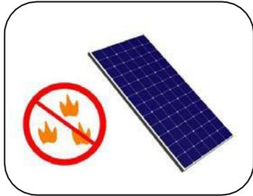
The module must not be installed close to fire or flammable materials.
