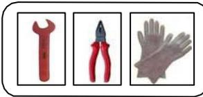
Make sure to use safety equipment (insulated tools, insulated gloves, etc.) when wiring.
